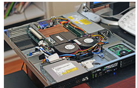
The inside and front of a Dell PowerEdge web server, a computer designed for rack mounting
