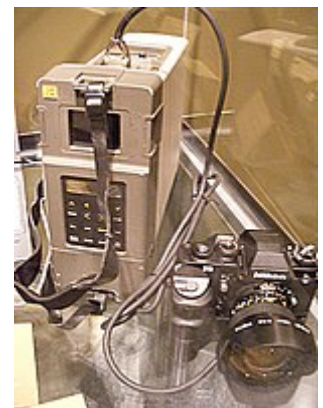
Kodak DCS 100, based on a Nikon F3 body with Digital Storage Unit
